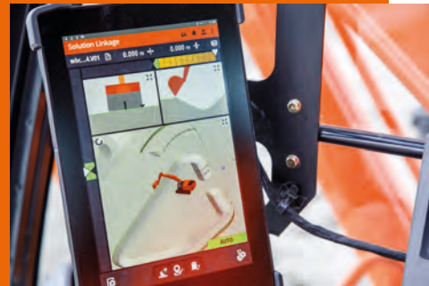
LEFT: The HMI monitor has a three-way split screen BELOW: Efficiency gains of up to 50% can be achieved with machine control
