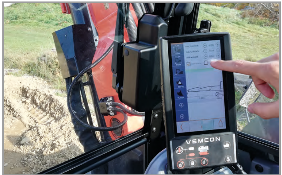
ABOVE: The Vemcon CoPilot automates and optimizes recurring machine movements
