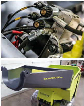
ABOVE: The electric steering and hydraulics are controlled by system application software
