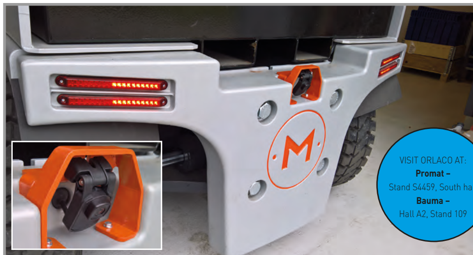
The Orlaco EMOS is a low-latency Ethernet camera compatible with onboard computer systems used in industrial vehicles
