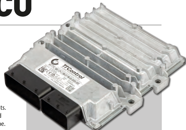
ABOVE: TTControl's HY-TTC 500 ECU family features SafeRTOS integration
