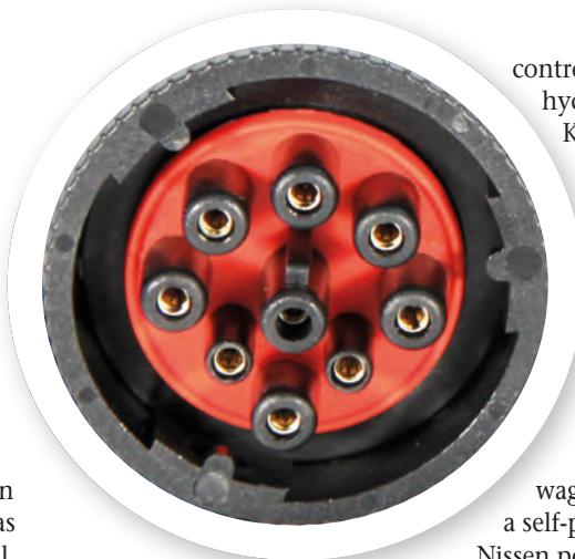
ABOVE: The standard ISOBus connector helps components from different manufacturers to work together
