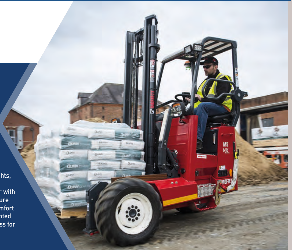
ABOVE: The M5's low hood, to the driver's right, maximizes visibility
