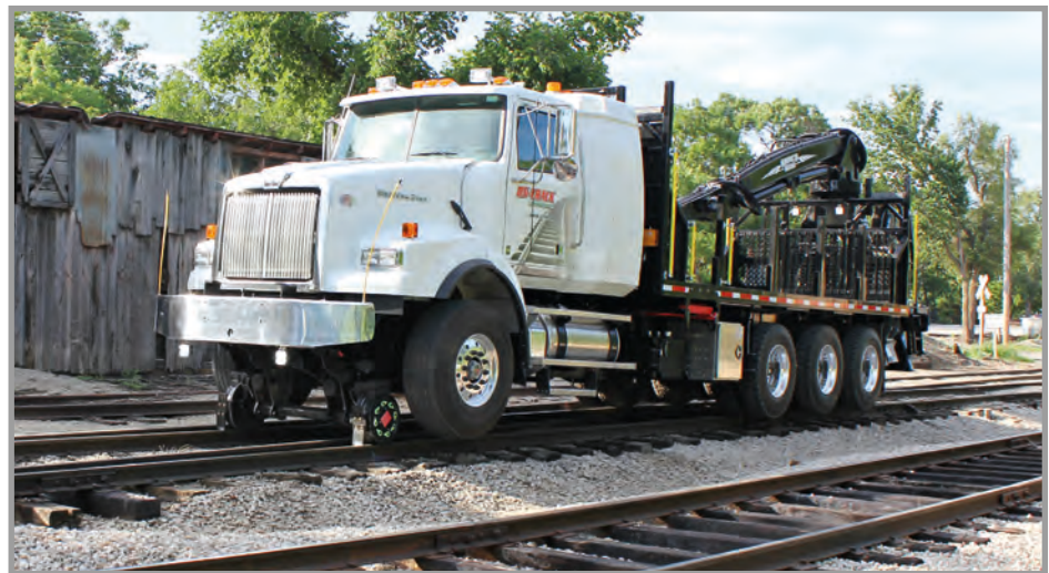
ABOVE: The CreepDrive system is designed for vehicles that operate at very low speeds
