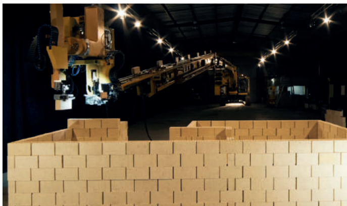
LEFT: The first prototype, the Hadrian 105, was built on an excavator frame, with bricks tracked down the boom
