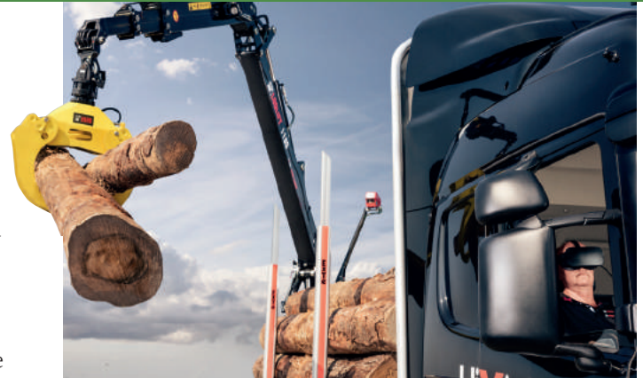
ABOVE AND BELOW: Hiab's HiVision virtual reality technology enables operators to remotely control forestry cranes from the comfort of their cab
