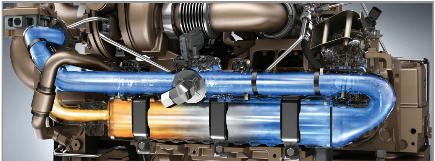
ABOVE: JDPS has developed an aftertreatment solution that is 20% smaller and 40% lighter than standard aftertreatments
