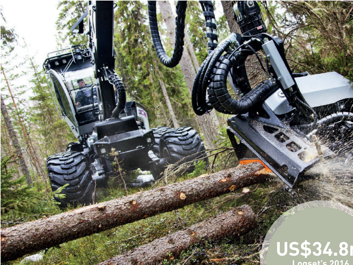
ABOVE: The Logset TH55 harvester head is suitable for use in clear-cut harvesting
