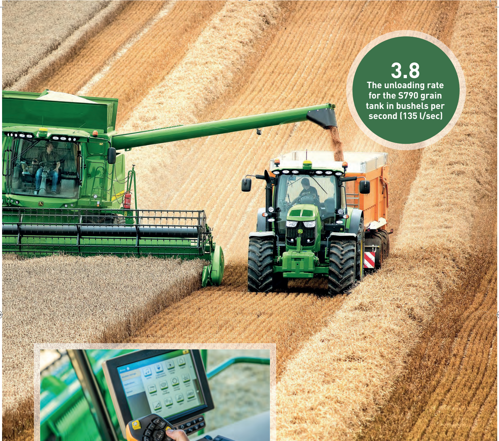
ABOVE: S700 combines are able to constantly monitor quality and cleanliness of grain LEFT: The 4600 CommandCenter is an app-based touchscreen display that's also found on John Deere tractors and sprayers
