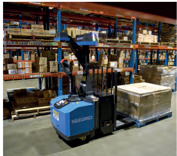
LEFT: Robot driver are here, but ones that look like this are certain to be confined to sci-fi movies for the time being BELOW: Seegrid's GP8 Series 6 in action
