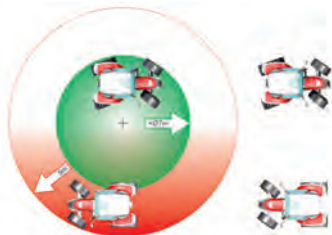
ABOVE: Maneuverability is at a high level thanks to the rear axle steering capabilities
