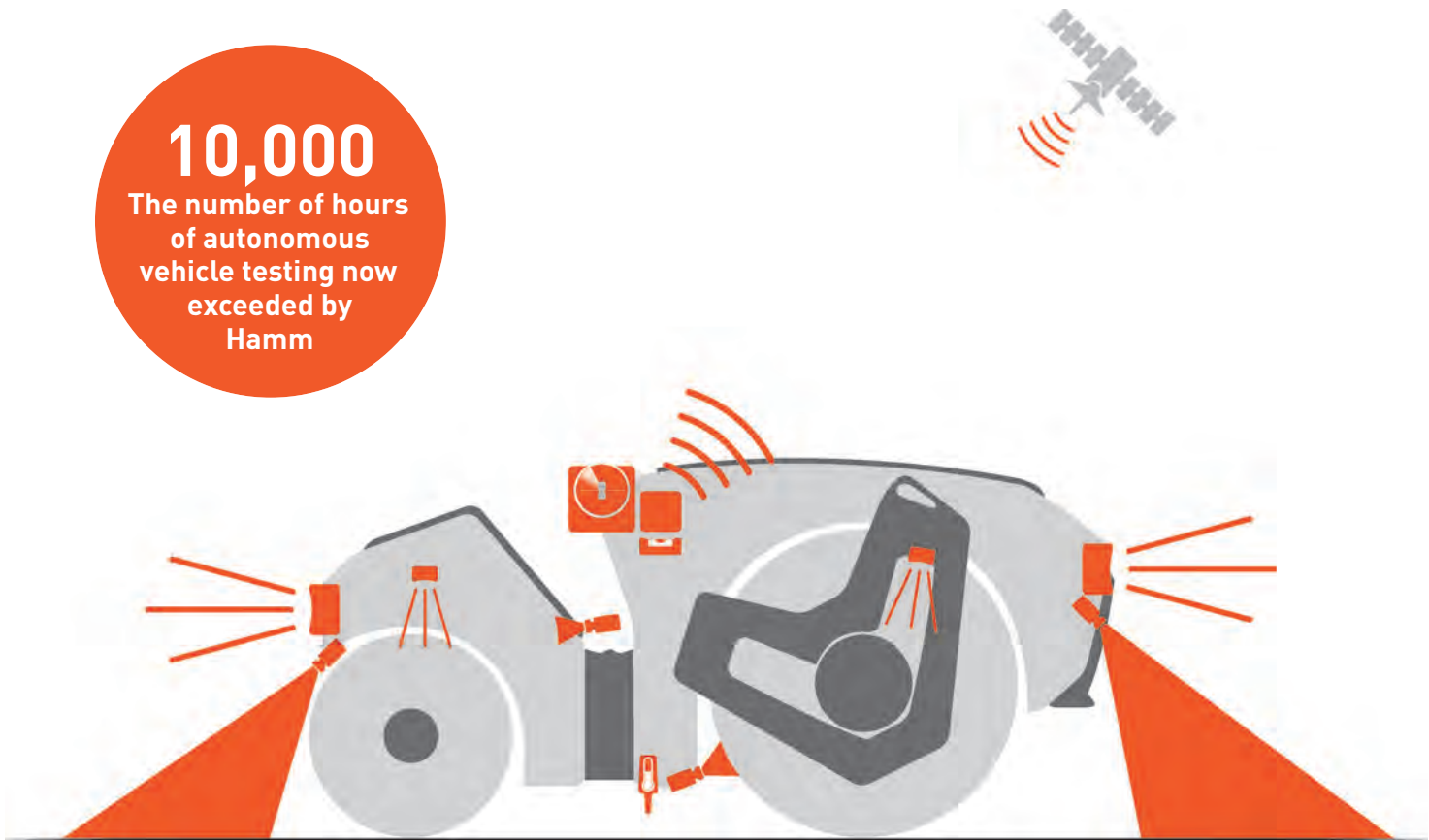
ABOVE: A self-driving roller requires numerous sensors such as radar systems, laser sensors, cameras, GNSS receivers, infrared sensors and incline sensors
