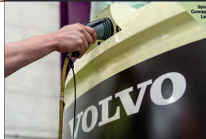
LEFT: The idea behind the EX2 is it gets charged up and then can run cable-free. However, it is possible to run it directly from a power source, too
