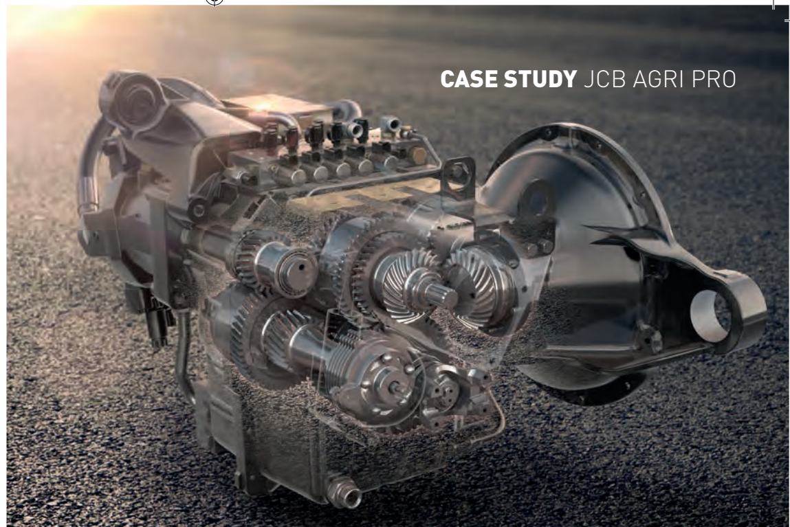
ABOVE: Inside the DualTech Variable Transmission gearbox, which is able to automatically switch from hydrostatic to powershift drive
