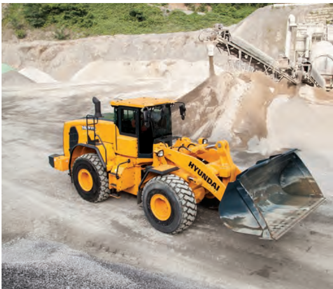
BELOW: The HL975 bucket is built with curved side plates to prevent material spilling and to protect the vehicle body
