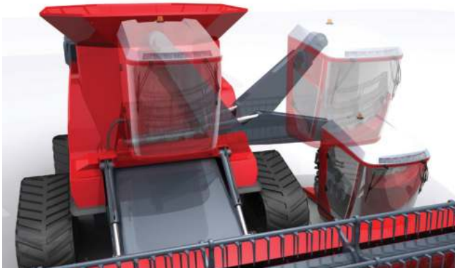
The cab swings down to ground level for ease of access; cab suspension is built into the boom
