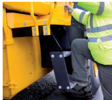
LEFT: Obese and aged operators alike would welcome lower step heights to simplify access to the machine
