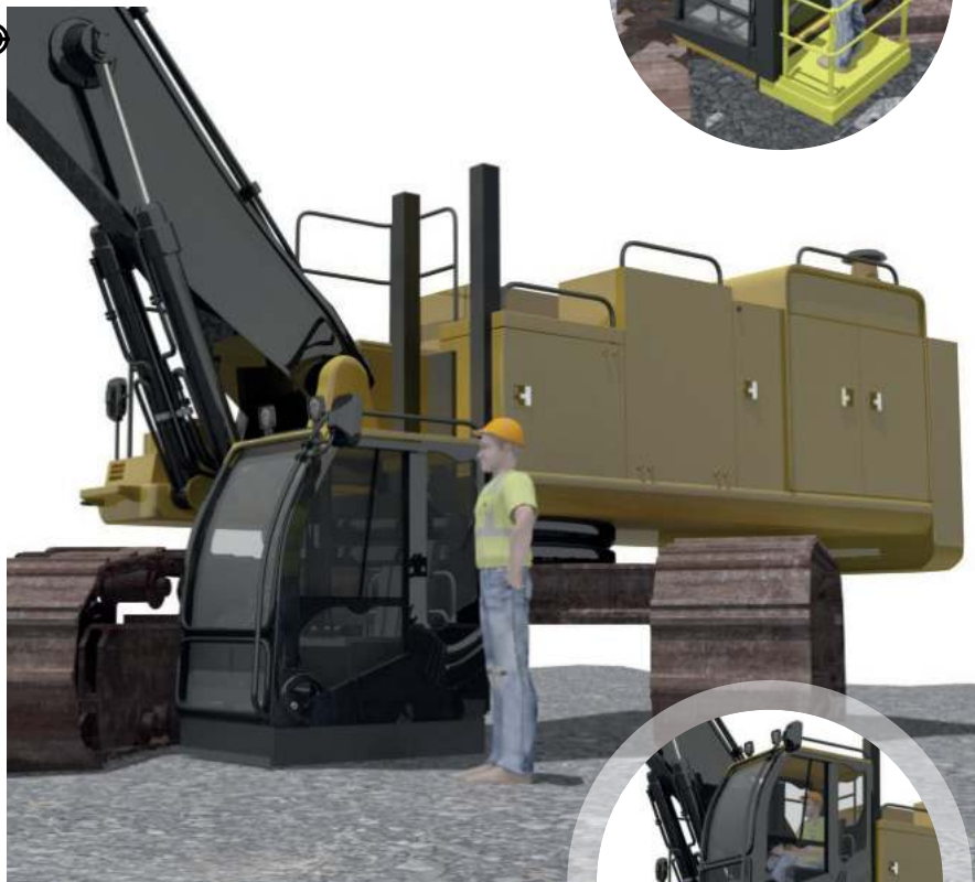
Using linear actuators, this solution only requires an operator to take one small step into the cab
