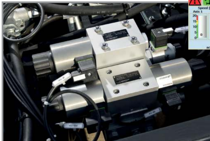
LEFT: Electronically controlled hydraulic drive and brake support
