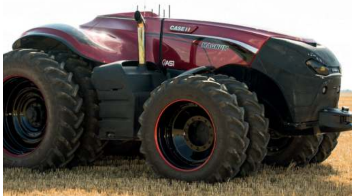
ABOVE: Case's Industrial Design Team re-imagined a Magnum tractor for a future autonomous era, eliminating the traditional operator station and crafting its sleek and dynamic lines
