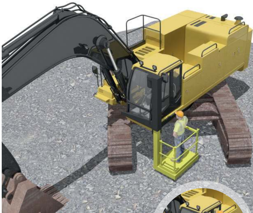
An ideal retrofit, the powered vertical lift relies on a single-post telescopic actuator
