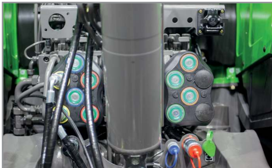
ABOVE: Neptune casting block with flat-face female couplings installed at the rear of the tractor
