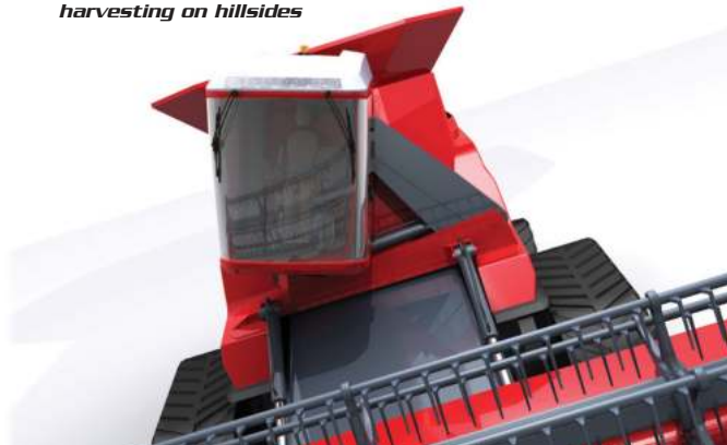
The cab's rotational ability is also useful for when harvesting on hillsides
