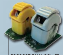
PROPORTIONAL ROLLER SWITCH WITH PWM DRIVER
