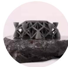
ABOVE AND BELOW: Planetary Resources and 3D Systems’ prototype object, made from a piece of an asteroid composed of iron, nickel and cobalt, using 3D printing
