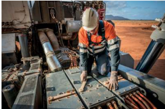
LEFT: The three frequency converter modules at the rear help reduce maintenance requirements as they can be easily removed and replaced
