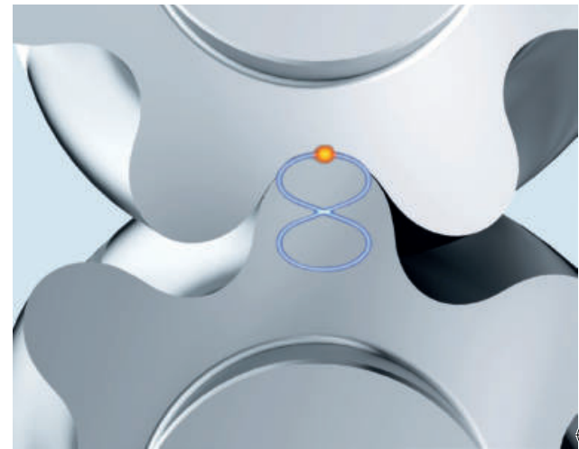
BELOW: The tooth profile provides zero-backlash continuous contact without any chambers of squeezed oil
