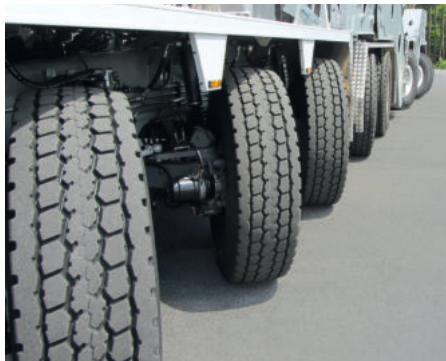
ABOVE: All eight axles are steered – two of them mechanically, and the other six via the electronic-hydraulic EHLA system
