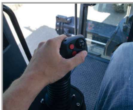
ABOVE: The Unigrip multi-axis joystick simplifies control of the notoriously difficult motorgrader
