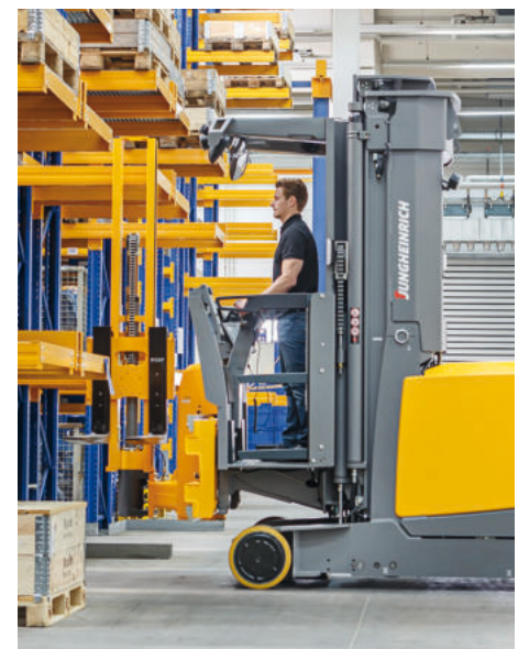
ABOVE: The EKX III offers the ability for the operator to control the load from the driver's cab up to a lift height of 14m
