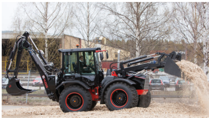
The steering system is a hydrostatic orbital control system with dual cylinders – digitally assisted by the wheels – in the center pivot with a steering angle of \pm 37^\circ and a frame oscillation of \pm 18^\circ
