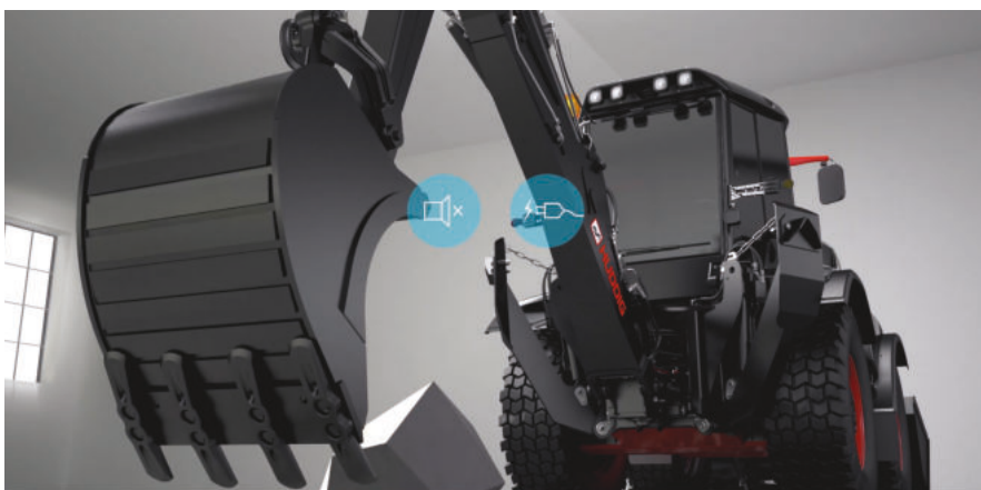
LEFT: The EMGs enable finer control of the working hydraulics, each delivering 30kW to enable silent operation when necessary
