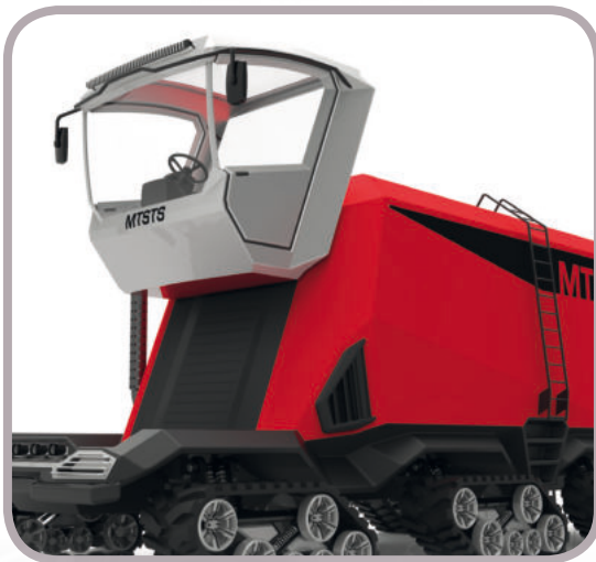
LEFT: The elevating cab provides an overview of the entire field
