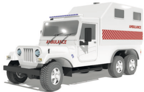
Even lightweight vehicles can be transformed for bigger duties with another axle
