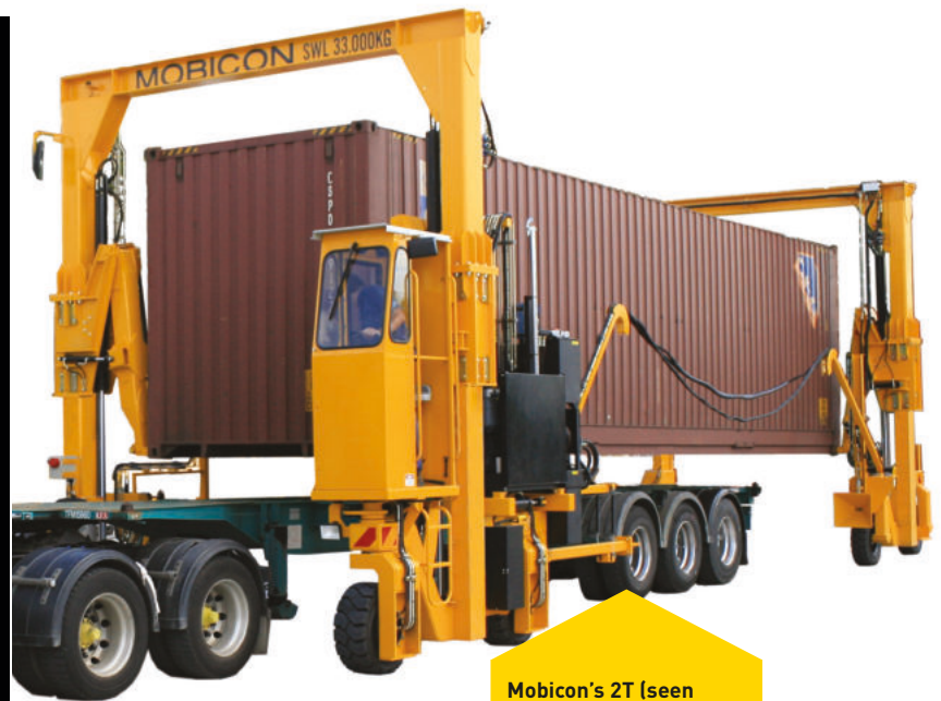
Mobicon's 2T (seen here transferring a container from a low loader) features four bogies that provide independent steering between front and rear
