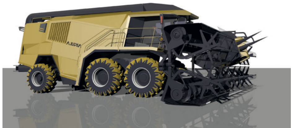
Convenient access to the cab is provided via ladders that wrap around the front wheels
