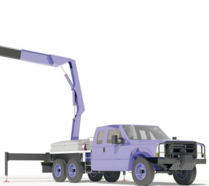
Big crane, small carrier - made possible by the third axle
