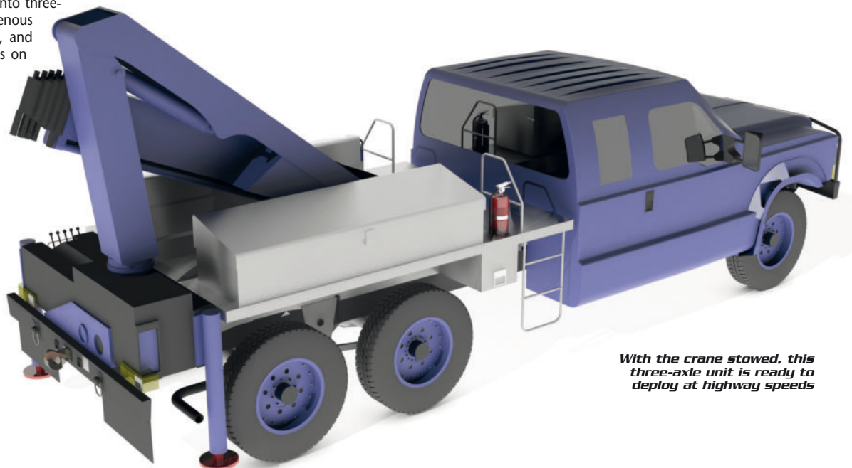
Even lightweight vehicles can be transformed for bigger duties with another axle
