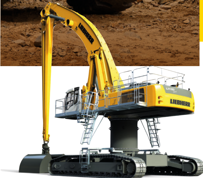
ABOVE: With a completely redesigned configuration, including angled 13m boom and straight 12m stick, the LH 110 C High Rise Port material handler features a hydraulic double-pivot cab with infinitely adjustable height and forward movement, and sliding doors with ground access. The patented energy recovery system (ERC) comes as standard
