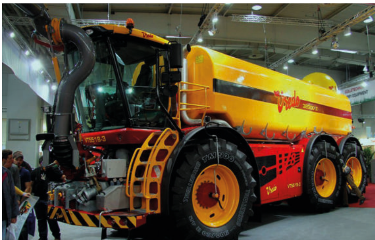
LEFT: A remote loading arm with gauge of 10in is positioned at the front of the machine, with material drawn in via a macerator-protected 12,000 l/min positive displacement pump
