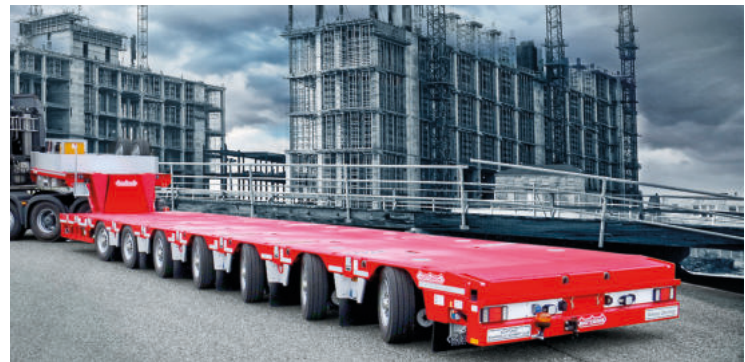
ABOVE: Nootboom’s pendulum axles provide just over 50% more suspension travel – up to 500mm – than a semi low-loader using other types of suspension
