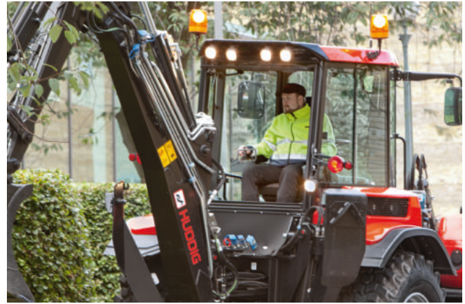
ABOVE: The driver cab has been designed with enhanced ergonomics and increased safety in mind. The buttons are ergonomically positioned and the joystick has a turnable ring making it possible to operate four functions with one joystick. The joystick console is stepless and adjustable and the control knob can be used for a chosen function, for example adjusting the hydraulic flow
