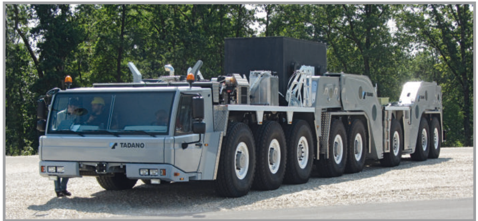
ABOVE: Tadano's ATF600G-8 – at 21.7m long, 3m in width and with eight axles, it has some demanding requirements in relation to maneuverability
