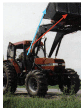
BELOW: Windshield height should be determined by the visual task, such as running a front loader at height, and the cab designed accordingly
