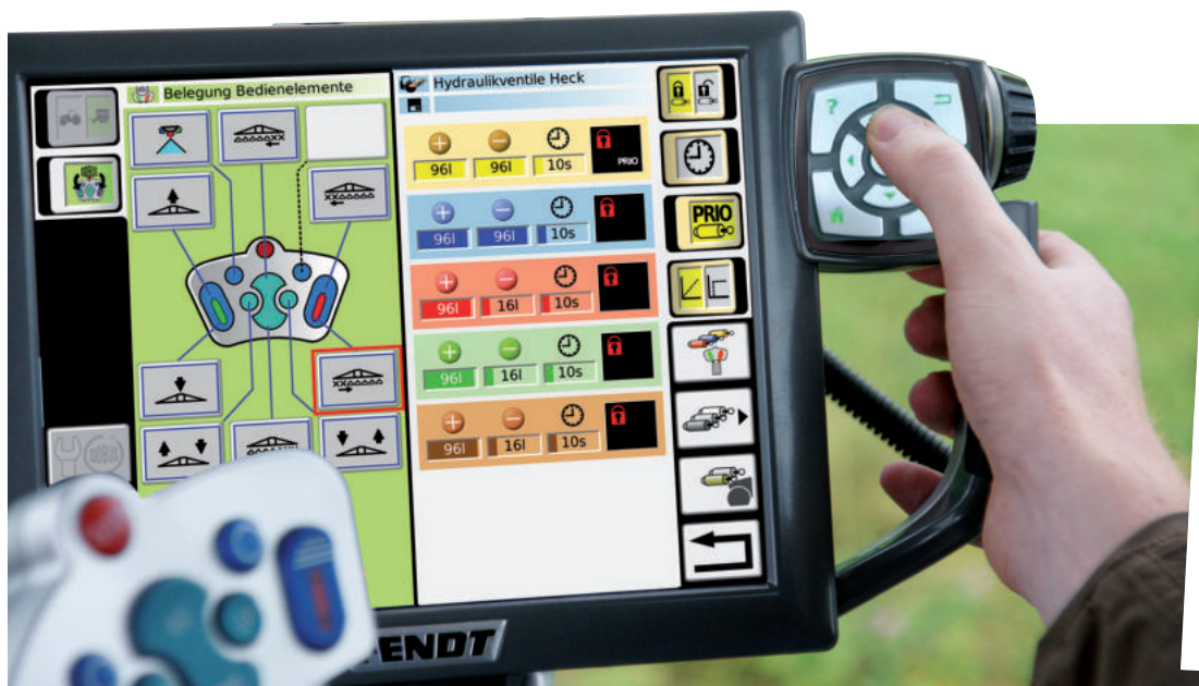
ABOVE: The Variotronic terminal is operated by touchscreen or keypad
