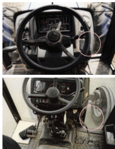
ABOVE: The top photo shows a tractor with a particularly wide front console; the lower photo shows how a tapered front console provides a clear line of sight to the ground around the front tyres – an especially important consideration in row-crop applications
