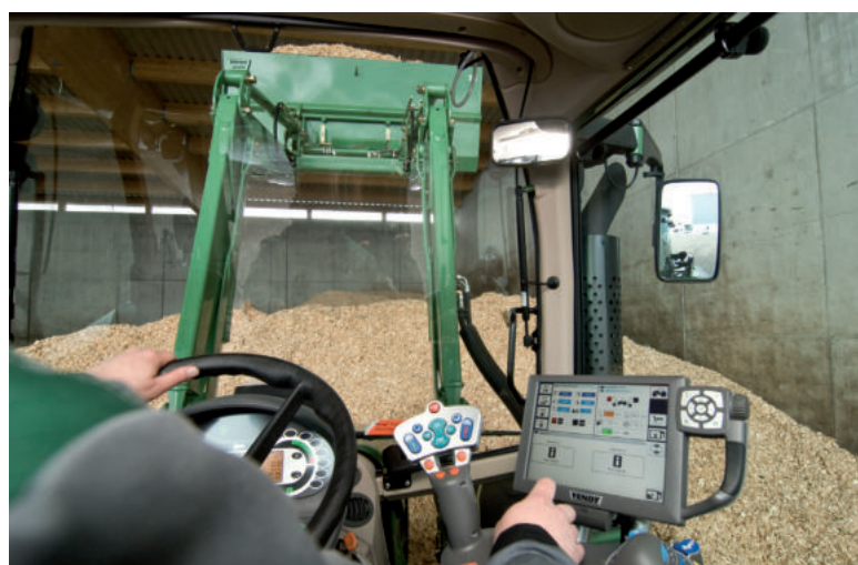
ABOVE: The Variotronic terminal is operated by touchscreen or keypad
