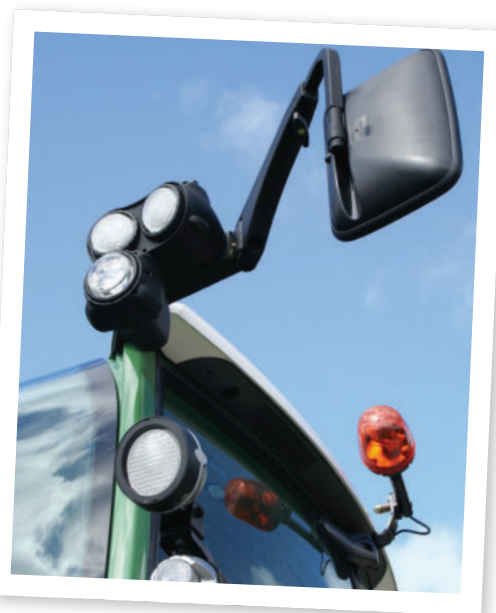
RIGHT: Worklights normally set into the roof panel find a new home in clusters with wing mirrors
