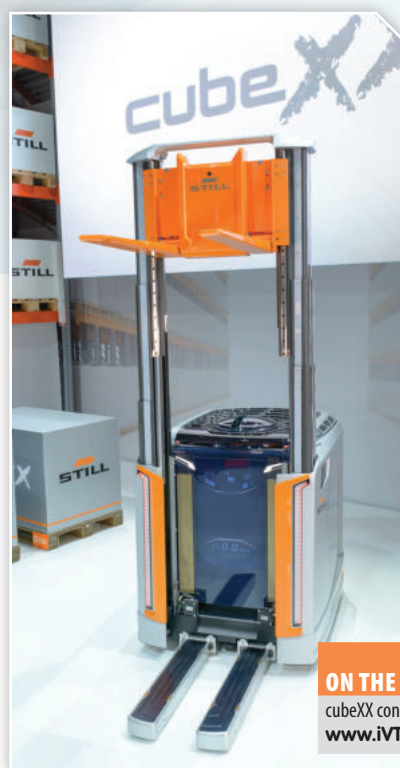
LEFT: The load supports ensure a safe stance for work as a high-lift pallet truck
