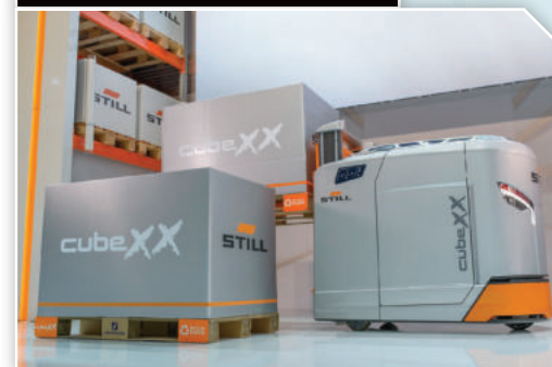
BELOW: The autolift function raises goods to a comfortable height while in order picker mode
