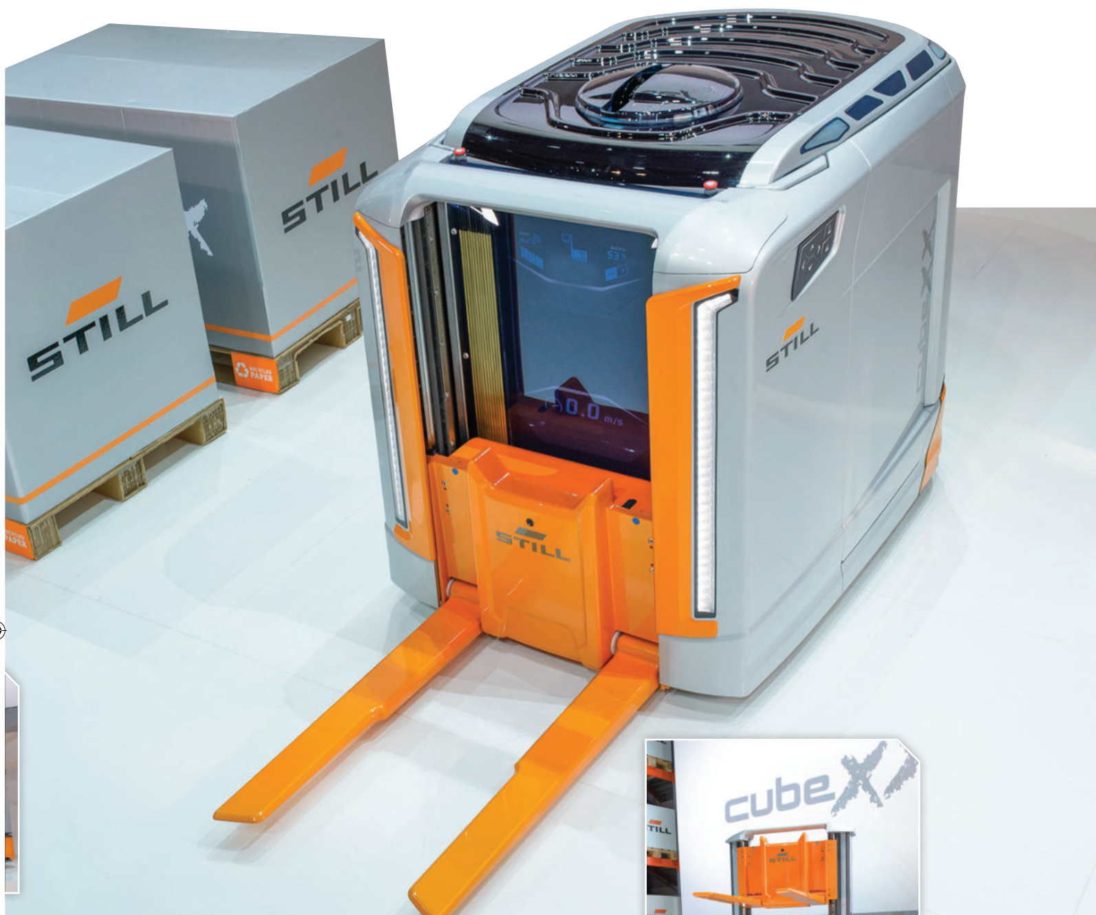
LEFT: The load supports ensure a safe stance for work as a high-lift pallet truck
