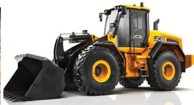
In its new type 457 wheeled loaders, JCB relies on MTU 6R 1000 engines with an output of 197kW
