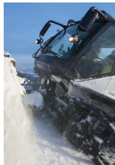
LEFT & ABOVE: The wider blade ensures greater thrust and makes the Leitwolf 45cm wider than other models in its class. Its teeth facilitate the breaking up of ice and snow and increases the efficiency of slope preparation
