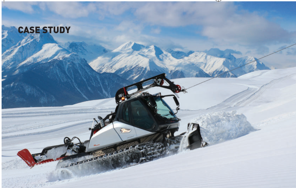
LEFT & ABOVE: The wider blade ensures greater thrust and makes the Leitwolf 45cm wider than other models in its class. Its teeth facilitate the breaking up of ice and snow and increases the efficiency of slope preparation
