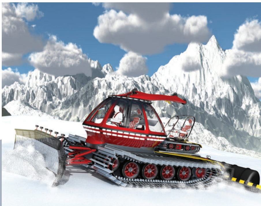
RIGHT: Driver's seat tilts up to 20° for more comfortable cross-slope operation
