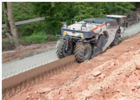
Wirtgen's cold recycler/soil stabilizer WR 200i, powered by an MTU Series 1100 six-cylinder in-line engine
