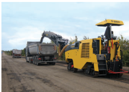
The 260kW MTU 6R 1000 is used in Bomag BM 1000/35 cold planers
