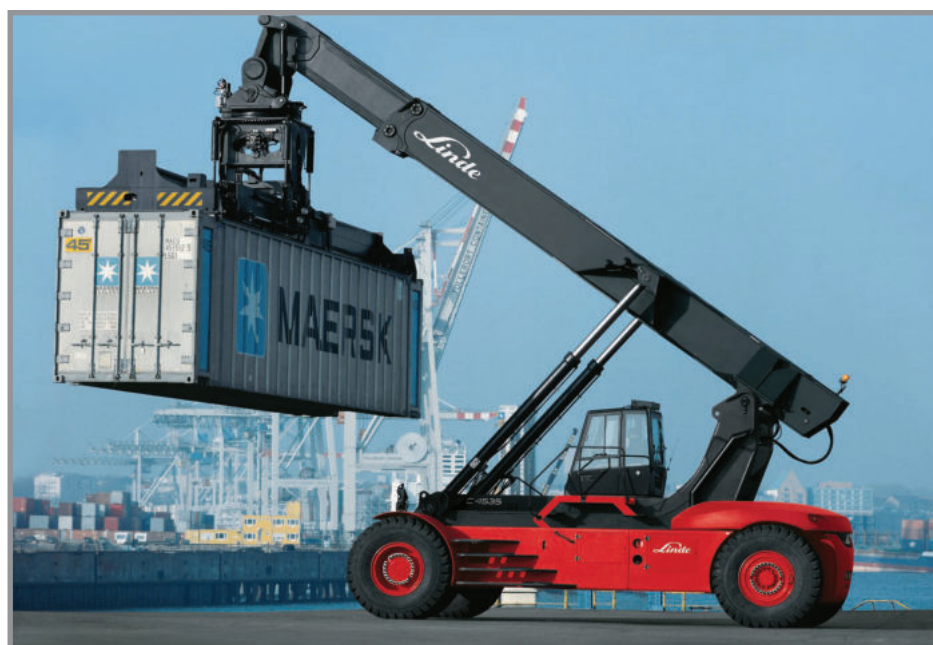
The impressive 80-ton reach stacker picking up an ISO container with ease, making it at home in ports around the world
